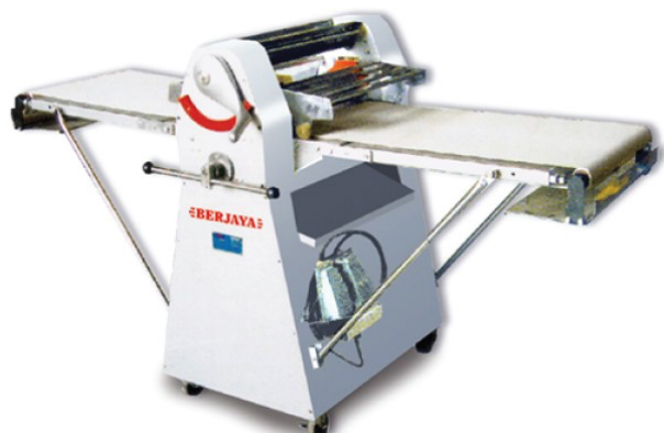
Dough Sheeter Conveyor Belt Wide(mm):500 Conveyor Belt Length(mm):2000 Voltage/Phase(V?Ph): 380-415/3
